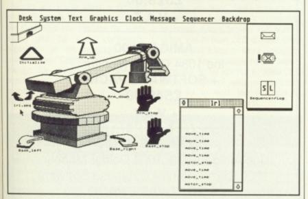
■ When you click on one of those icons a message is sent to the robot. These messages can be strung together in sequences and executed in one go. Hence the robot can perform mundane tasks indefinitely.
