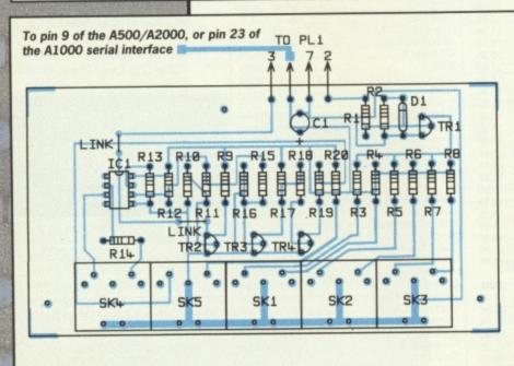
■ Figure 1 - The component layout. In blue are the conductive copper tracks on the board. What you have to do is insert each component into its correct holes from the uncoppered side of the board, so that the wires stick out of the coppered side. Then solder the leads to the tracks. Refer to the parts list to make sure you put the right ones in the right places.
