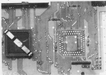
■ Take this to your dealer. There are 68 holes to desolder before you can fit the blitter socket. And a further two (W3 and W4) after. But first you've got the protective shielding to contend with.
