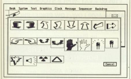
■ The 20 icons that can be added to the backdrop. Icons can have commands attached to them which tell motors and other components to perform certain jobs. For instance, a motor can rotate in a given direction at a given speed.
