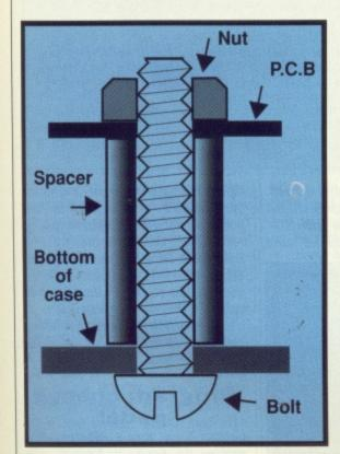
■ How to mount the board in the box using spacers. Drill out the three mounting holes marked on the board if you need to – don't try a hammer and nail or you'll split it!
