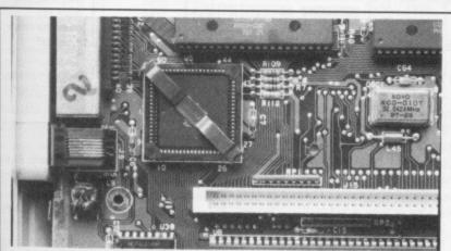
■ 4 - Now fit the chip. The blitter socket has a tiny hole bored into one of its edges; the blitter has a similar-sized indentation along one of its sides. This indicates which way the chip fits into the socket. Put the bar back when you've fitted the blitter. And now put the rest of the ST back together. Pray that the blitter functions correctly.
