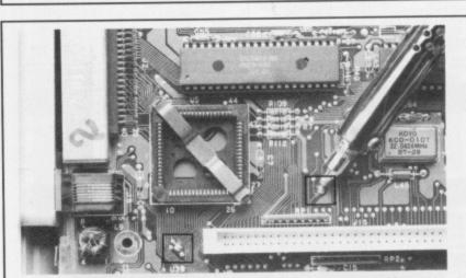
■ 2 – You'll find the empty blitter socket to the right of the cartridge port and above the 68000 processor. Look for two relatively large solder blobs. One can be found above a resistor pack (RP1) while the other is left of the internal hard disk socket. Hope you've brought a solder sucker with you.
